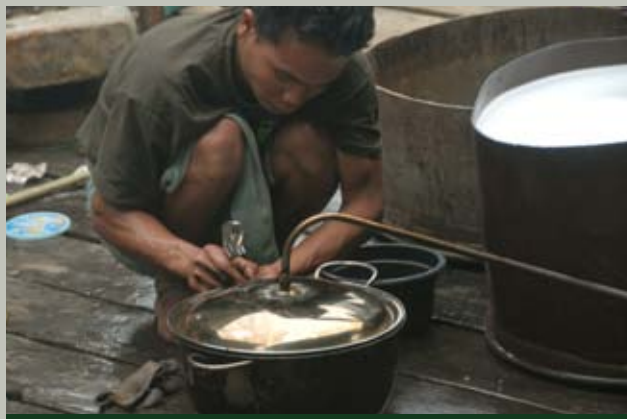
Gold worker tests a new, large retort to prevent mercury loss to the air
